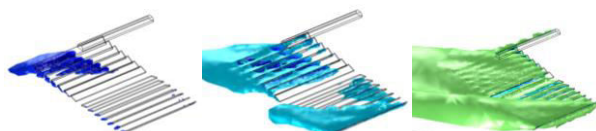
Fig.5. Wind velocity isosurfaces at 7m/s, 14m/s and 21m/s respectively
