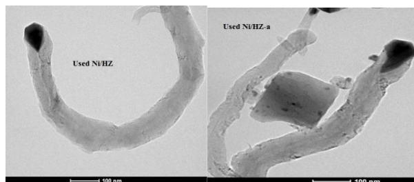
Fig. 7 TEM images of used catalysts in CDM at 520 °C for 4 h.
