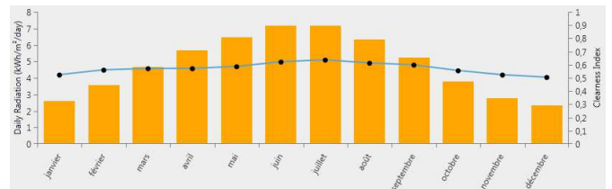
Fig. 3 Monthly average solar global horizontal irradiance (ghi) data. the annual average (kWh/m 2 /day) is 4. 80.
