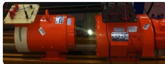
Fig.5. Experimental test rig: Asynchronous generator(4,5 kW), DC motor (3kW)
