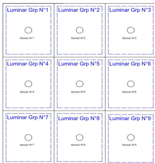
Figure.10. Distribution of sensors and luminaire groups inside the greenhouse
